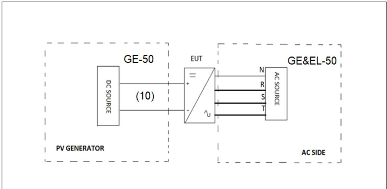
Different equipment has been used to take measures as it shown in chapter 2.4. Current and voltage clamps have been connected to the inverter input / output for all the tests.
